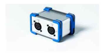
The **Pan Con Passive converter** is required for connection audio signals and control signals to a Pan Beam network. The Pan Con V3 Passive converter have two XLR audio connections for audio signals and a two wire phoenix connector to fed RS 485 control signals. Those devices are equipped with an alarm contact, which allows the automatic transmission of status notifications from the Pan Beam's network.
